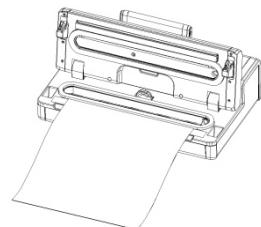
Put one end of the bag on top of the sealing bar, but not enter the vacuum chamber.
