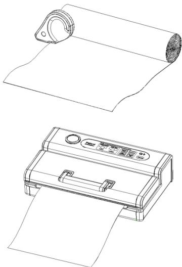
Roll out the bag roll to the desired length and cut with a bag from the roll with the cutter.
