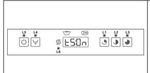
"on" = **the minimum temperature of rinse** as set, independently from the intake water temperature, the nominal duration of cycle may be extended by a few seconds.
