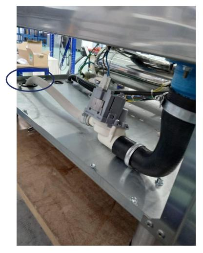
Drain hose is a white and longest one. As explained earlier, the right side of the white hose should be connected to the drain pump and the left (other) side of the hose should be extracted to the outside from the biggest left hole in the body as in the picture.
