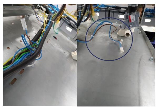
You will find the cable group and there are two cables, blue and brown which have a white connection head or on the cables it is written either Drain Pump or Drenaj Pompası in Turkish. Extend the blue and brown cable from its place to connect the drain pump.
