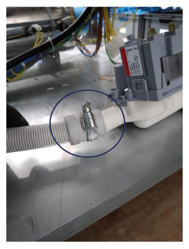
Left side of the drain pump has also connection to the hose. The white slim hose should be connected to the drain pump and must be well tightened with hose clamps.
