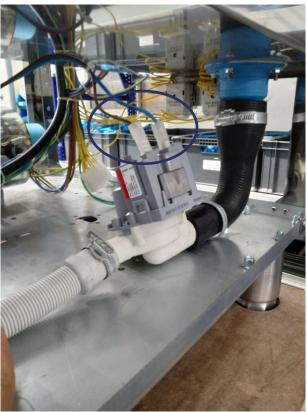
As shown in the picture, the drain pump has two connection channel top of it. So, the blue and brown cables connected to that channel. However, the color of the cable and place of the connection (right and left) can be connected randomly.
