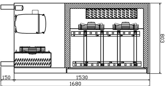
A: Please follow the instructions, properly install and place the equipment, properly connect the water supply pipe, drain pipe, and reserve additional space 10cm at the installation site to meet the installation requirements. (Air cooling equipment needs more space to meet the air flow and heat discharge.)
