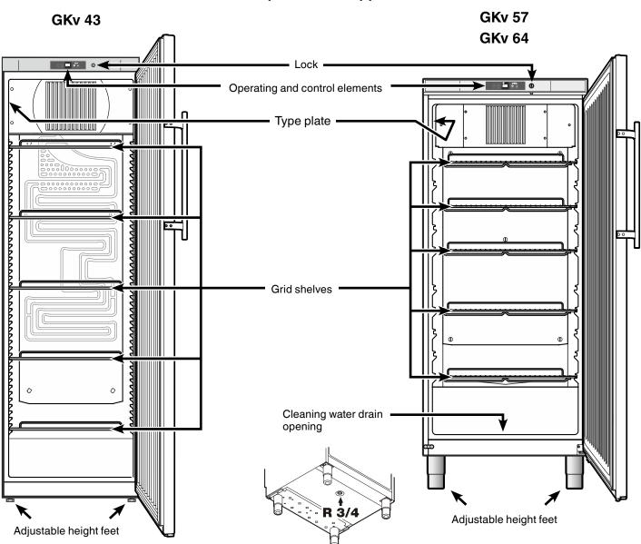
A drain hose with an R 3/4 connection can be fitted to the underside of the appliance.
