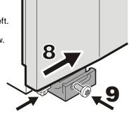
4. Transfer lower hinge bracket and cover plate to the opposite side.
