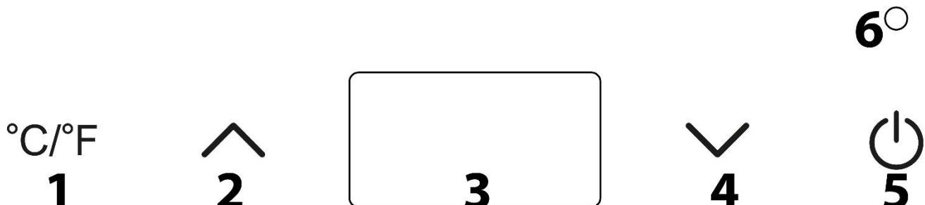
1 Change from °C to °F, as well as display of the current temperature inside the wine bottle cooler
