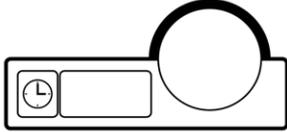
Turn rotary knob to set the cooking time of the selected cooking mode from 0:00 minutes to 24.0 hours. Turn left for \* ---\* continuous operation.
