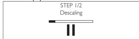
The first descaling phase starts. Press the "OK" button to pause the operation. Press the "OK" button again to resume the operation. When the solution in the tank is finished, the machine requests to empty and rinse the tank with fresh drinking water.
