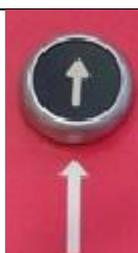
Once the bowl trolley has been correctly inserted into the lifter forks, this button is used to raise the bowl to the discharge position to allow the dough to be emptied out.
