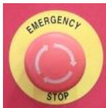
All lift operations can be stopped by pressing the emergency button (position 3).
