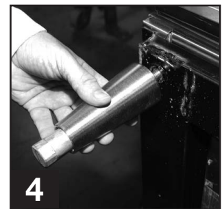
4 Thread leg into cabinet bottom frame rail.
