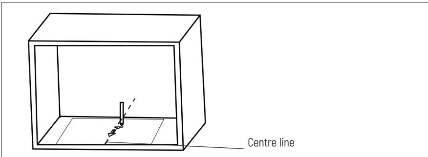
3. Remove the bottom cabinet template and fix the mounting plate with screw A.
