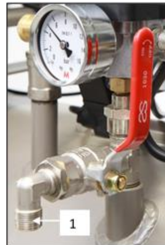
Fig. 8: Connecting to the compressed air outlet
