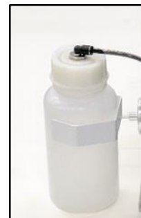
Fig. 16: Check of the condensate collection vessel
