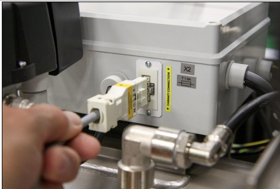
Fig. 13: Connect the cabinet to the compressor
